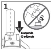
1. The liquid volume of the gas replenished : the main machine must be turned off before replenishing the gas, and after replenishing, the receiver; can be started. Align the aeration tank to the device, with the gaspin perpendicularly fixed, and press and hold the aeration tank into the gas adding hole for 10 seconds.
