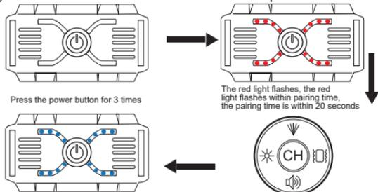
The blue light will stay on 5s after the successful pairing, and the buzzer emits two beeps at the same time
