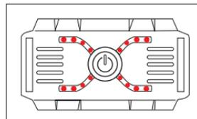
Receiver low voltage hint: when in low voltage state, The red light flashes five times every ten seconds
